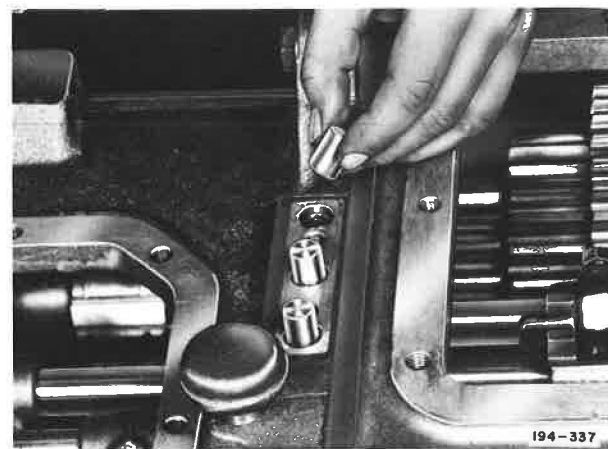
Figure 5-215. Installing Shift Rail Poppet Ball Pins (Early Production Units Only)
