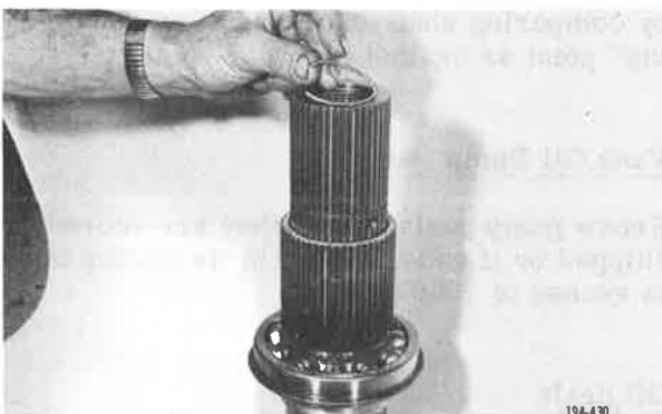
Figure 5-602. Removing Roller Bearing Retaining Snap Ring
