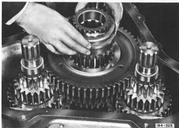
Figure 5-131. Removing First Speed Sliding Clutch
