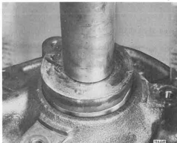
Figure 5-911. Pressing Seal into Cover
