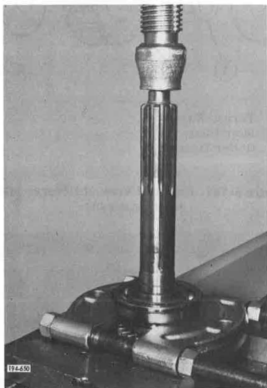
Figure 5-740. Pressing Bearing Off Shaft
