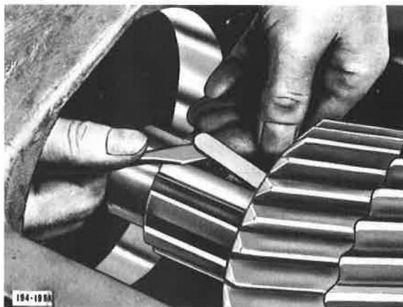
Figure 5-11. Removing Fourth or Fifth-speed Gear Sleeve Key
