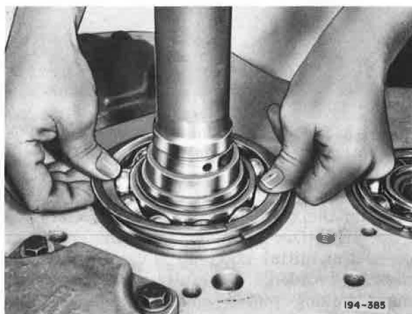
Figure 5-172. Installing Compound Main Driving Pinion Ball Bearing Positioning Snap Ring
