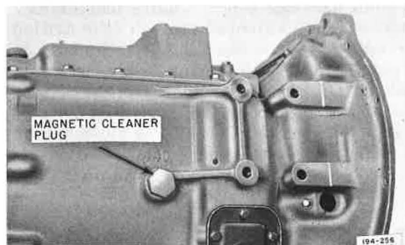
Figure 5-4. Typical R.H. Side of Case Location of Magnetic Oil Cleaner Plug
