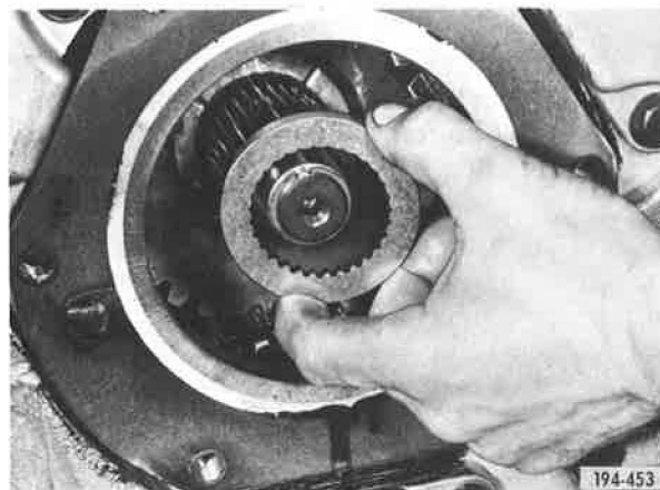
Figure 5-104. Installing Fourth Speed Gear Selective Thrust Washer
