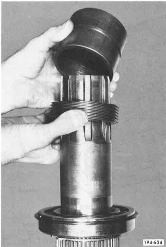
Figure 285. Installing Gear and Spacer
