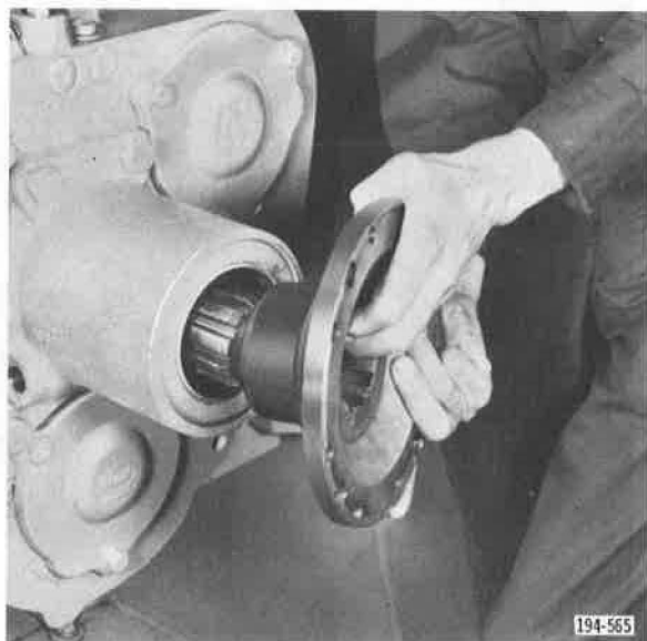
Figure 391. Installing Drive Flange
