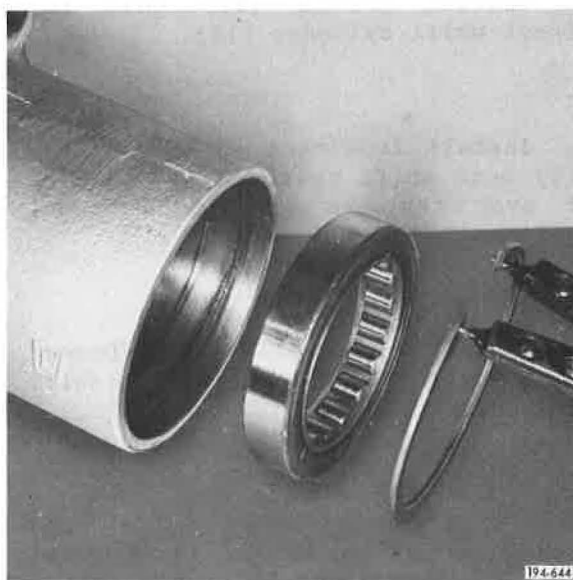
Figure 275. Installing Bearing and Snap Ring
