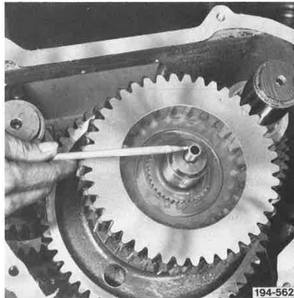
Figure 49. Mainshaft Oil Tube
