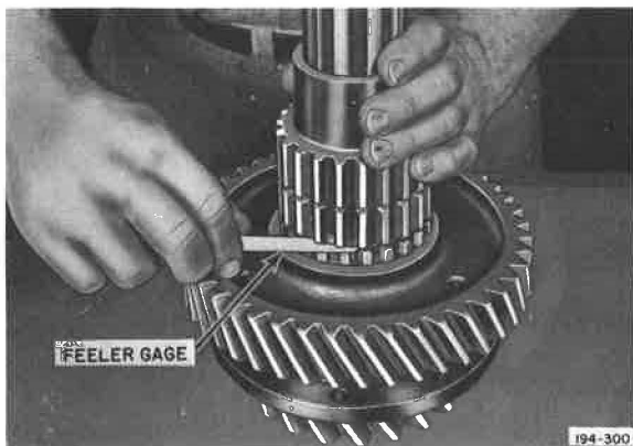
Figure 5-17. Method of Checking Gear End-play
