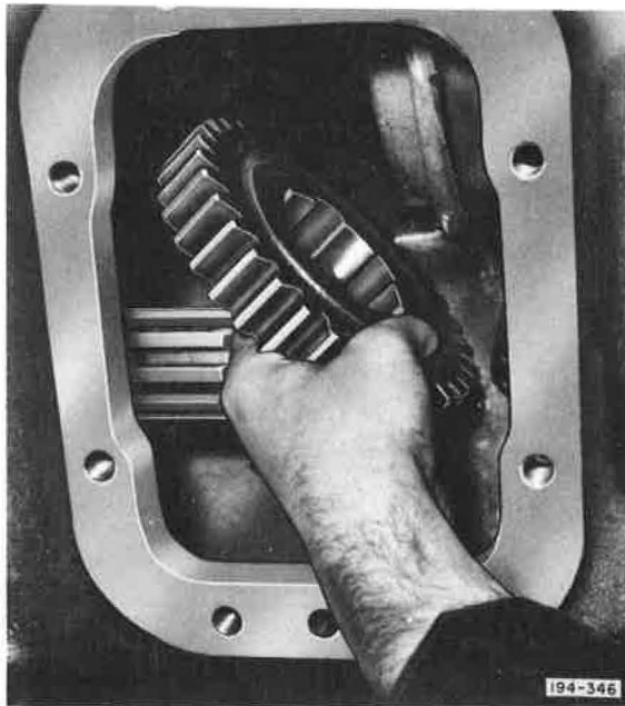
Figure 5-6 . Installing Right-Hand Power Take-off Gear Through Lower Power Take-off Opening
