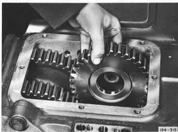
Figure 5-128. Removing Fourth Speed Gear
