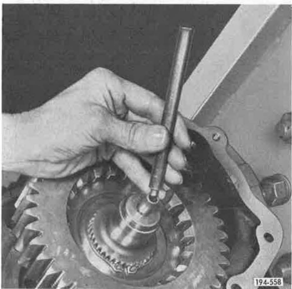
Figure 5-967. Installing Oil Tube
