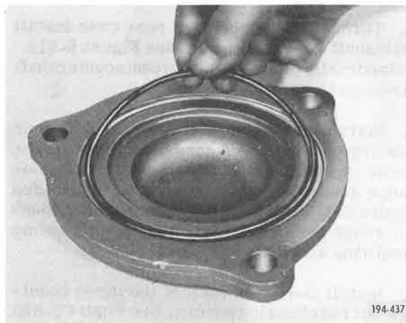
Figure 5-620. Installing Rear Countershaft Rear Bearing Cover O-ring
