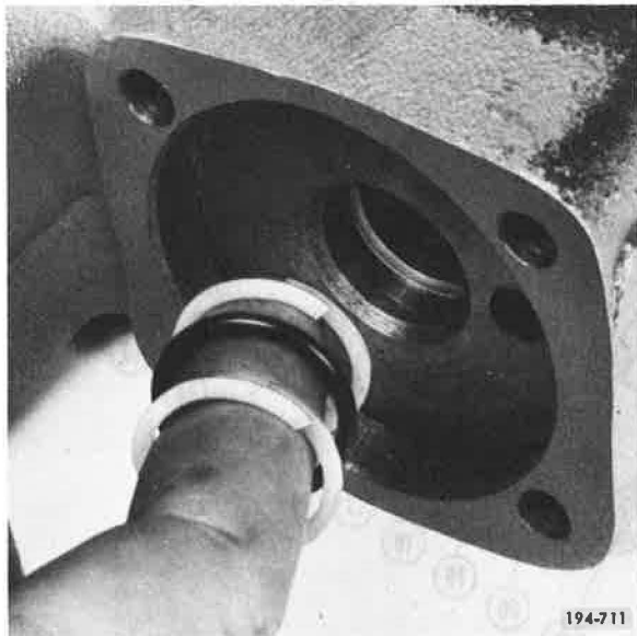
Figure 231. Installing O-Ring and Teflon Rings
