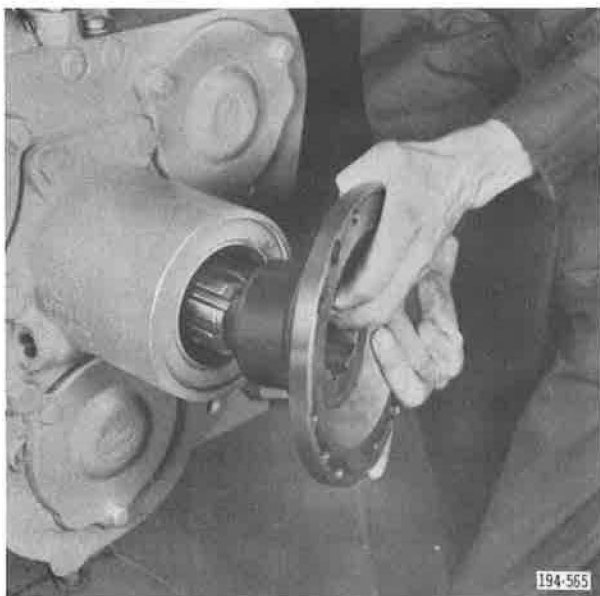
Figure 5-533. Installing Drive Flange
