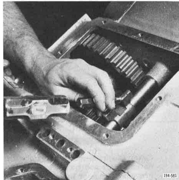
Figure 5-242. Driving Shift Rail Forward
