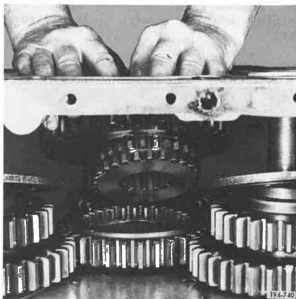
Figure 93. Removing Sliding Clutch and Lo-Range Gear
