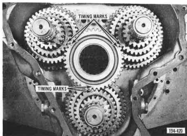
Figure 5-629. Front Mainshaft Third Speed Gear Temporarily Installed
