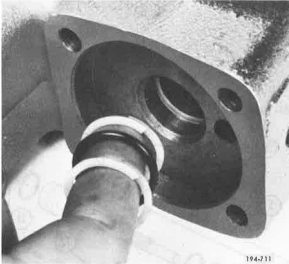
Figure 5-406. Installing O-ring and Teflon Rings
