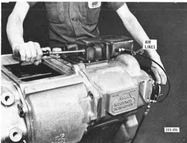
Figure 5-656. Adjusting Direct and Lo-Range Shifter
