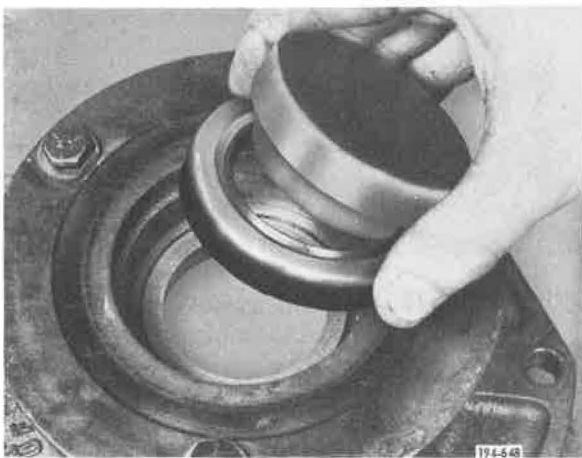
Figure 5-468. Placing Seal in Position
