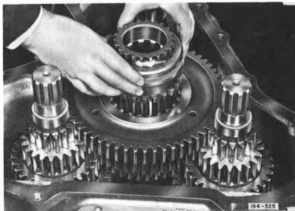
Figure 5-44. Installing First Speed Sliding Clutch
