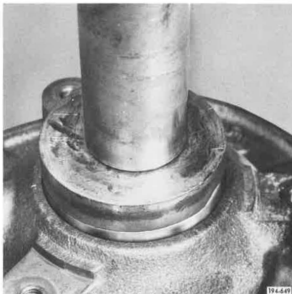
Figure 315. Pressing Seal into Cover
