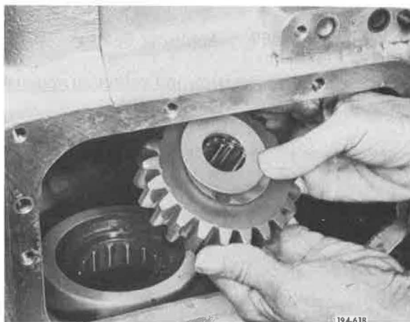
Figure 5-475. Installing Reverse Idler Gear Assembly
