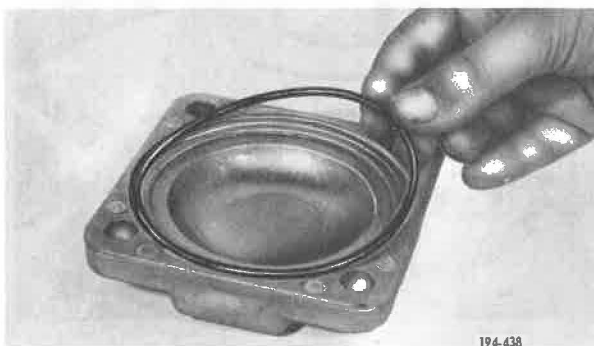
Figure 5-633. Installing Front Countershaft Front Bearing Cover O-ring
