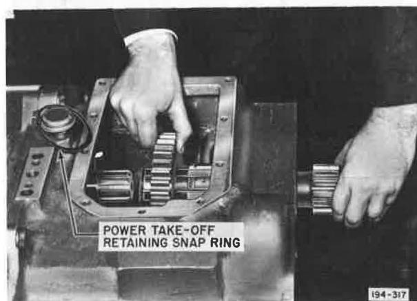
Figure 5-45. Installing P. T. O. Gear on Rear Countershaft
