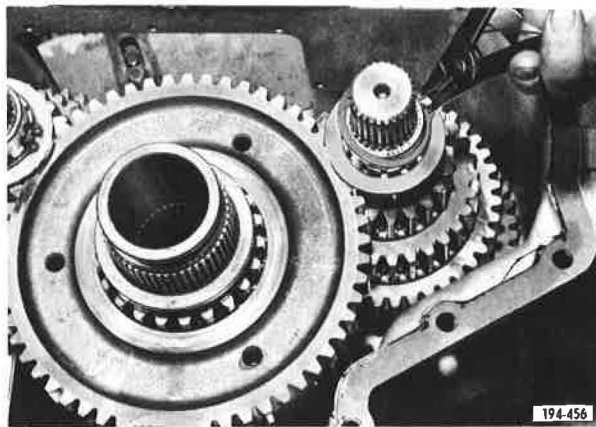
Figure 5-79. Removing Thrust Washer Retaining Snap Ring
