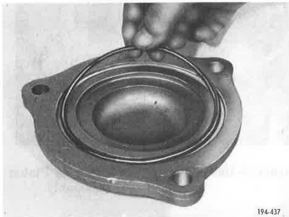
Figure 5-101. Installing O-Rings in Rear Bearing Cover
