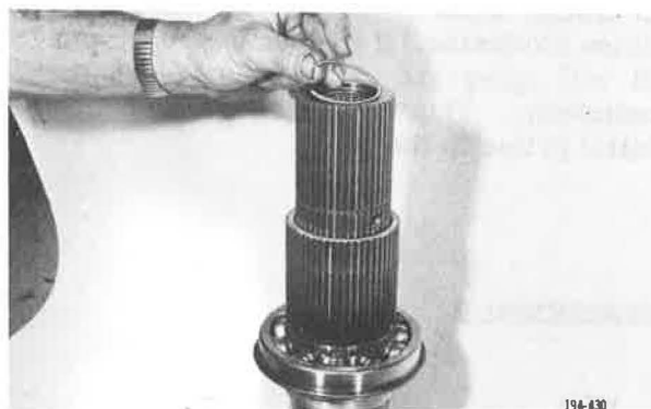
Figure 5-608. Installing Front Roller Bearing Snap Ring
