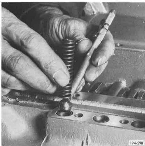
Figure 413. Installing Poppet Balls and Springs
