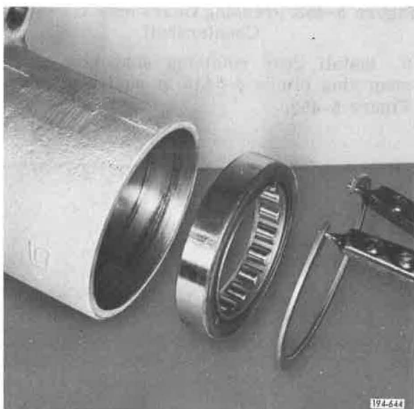
Figure 5-448. Installing Bearing and Snap Ring
