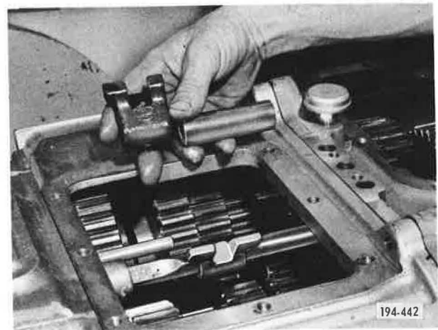
Figure 5-653. Installing First Speed Shifter and Reverse Speed Lockout Spacer
