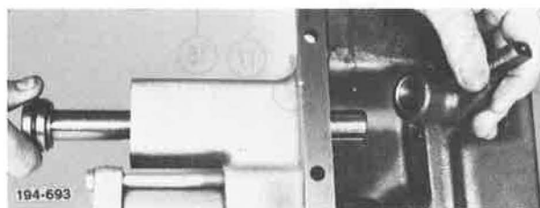
Figure 5-421. Installing Shift Rail and Shifter
