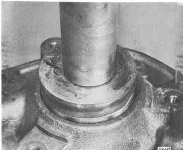
Figure 5-469. Pressing Seal into Cover
