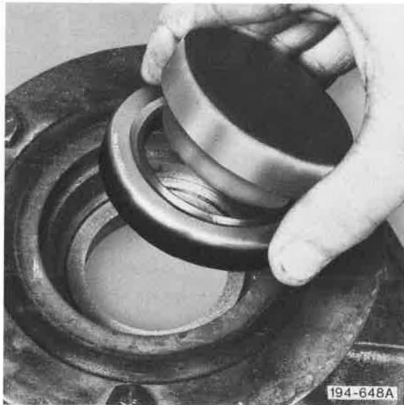
Figure 314. Placing Seal in Position
