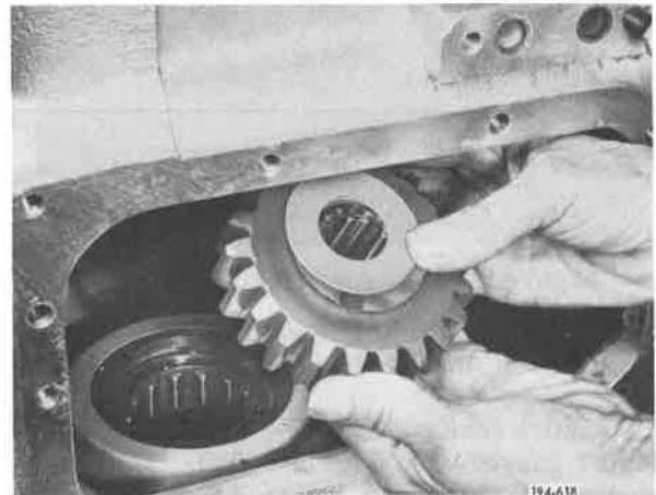
Figure 5-917. Installing Reverse Idler Gear Assembly
