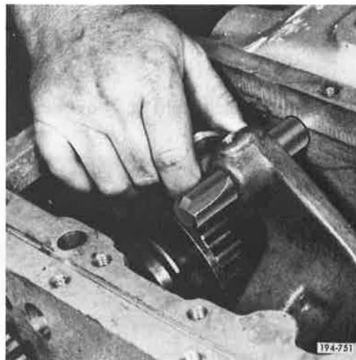
Figure 22. Removing Shift Rail
