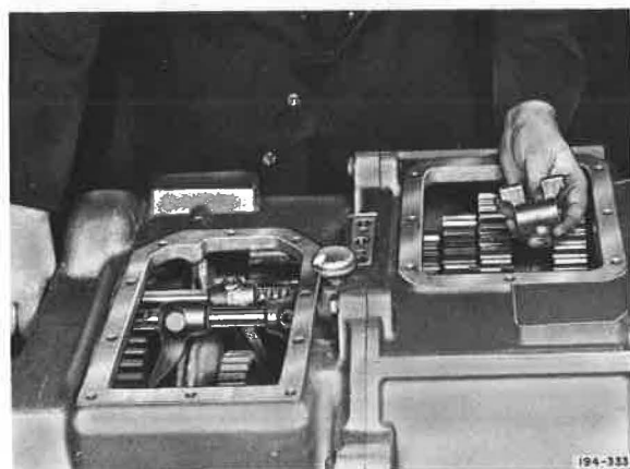
Figure 5-60. Installing Second and Third Speed Shifter
