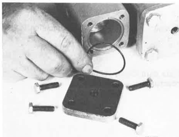
Figure 5-327. Removing Cover and O-ring
