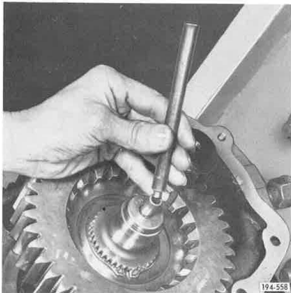
Figure 363. Installing Oil Tube
