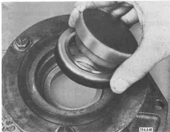
Figure 5-910. Placing Seal in Position
