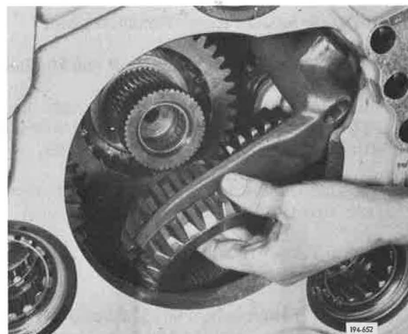
Figure 5-496. Installing Sliding Clutch and Shift Fork
