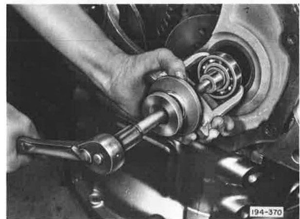
Figure 5-147. Removing Compound Countershaft Rear Bearing
