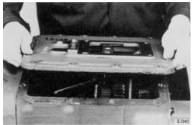
2. Jar to break the gasket seal and lift the shift bar housing from transmission.
