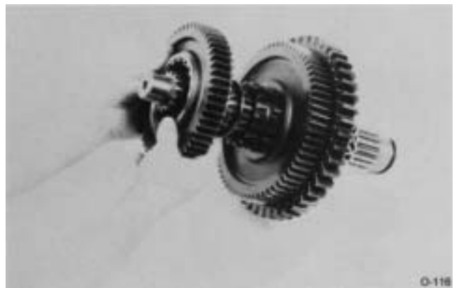
8. Remove the 3rd speed gear and spacer from front of mainshaft. The 3rd speed gear limit washer cannot be removed at this time as it is
