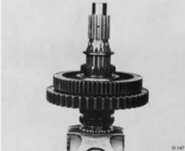
16. Reposition mainshaft assembly in vise, pilot end up.
