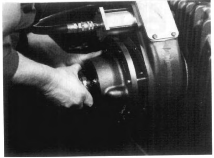
FIG. 6.7-9 With air applied to shift cylinder, align clutch gear on declutch output shaft with internal gear teeth on clutch collar and assemble carrier with gasket to the opening of the declutch housing. Tighten 8 mounting bolts to the appropriate torque.
