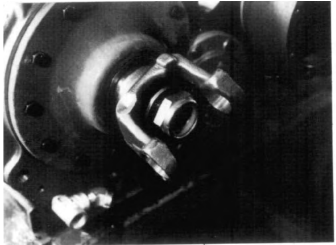
FIG. 6.4-19 Examine yoke or companion flange hub diameters for nicks or sharp corners, remove with emery cloth. Grease seal diameter and carefully slide hub into seal, using extreme caution not to damage seal lips.
