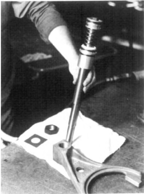
FIG. 6.6-1 Assemble shift shaft with small O-ring, adapter tube with O-rings, spring, stop ring, piston with O-rings, lockwasher and locknut together as shown.
