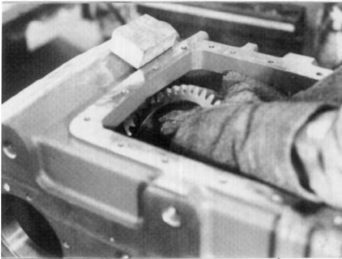
FIG. 6.2-1 Place upper shaft gear in heater for approximately 15 minutes. Add upper shaft bearing cones for last 3 minutes of heating time. While gear is heating add key to upper shaft.
