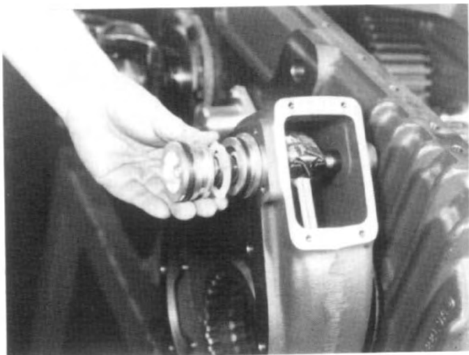
FIG. 6.7-7 Assemble shift components as shown and indicated in shift shaft assembly section. Add cover plate.
