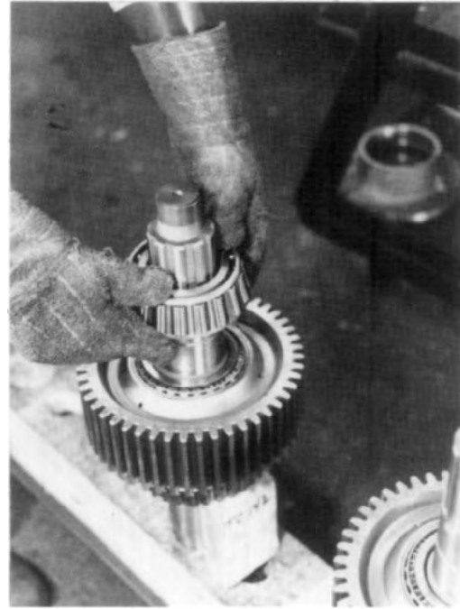
FIG. 6.3-7 Place shaft bearing in heater for 3 minutes, then slide over shaft.
