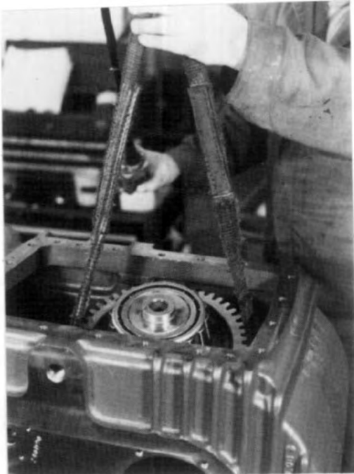
FIG. 5.1-17 With sling or lifting device remove intermediate shaft from housing.
