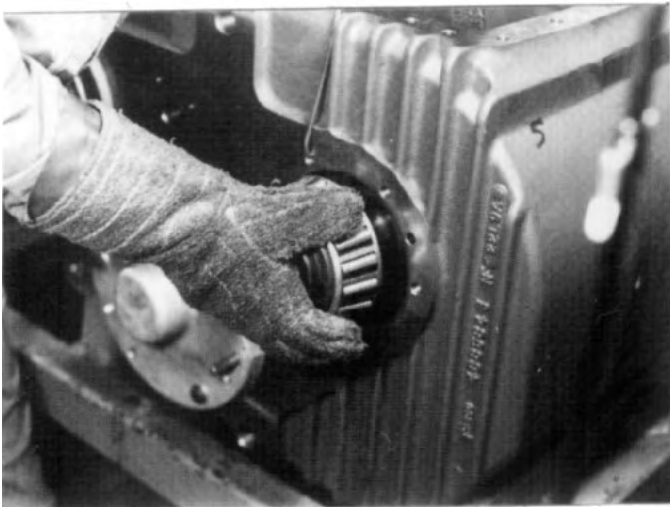
FIG. 6.4-6 Heat remaining shaft bearing cone in heater for approximately 3 minutes and with heat resistant glove slide bearing on shaft to butt against bearing cone under gear.
