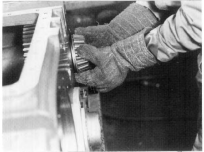
FIG. 6.2-3 Still wearing gloves quickly assemble bearing cone to rear of upper shaft.
