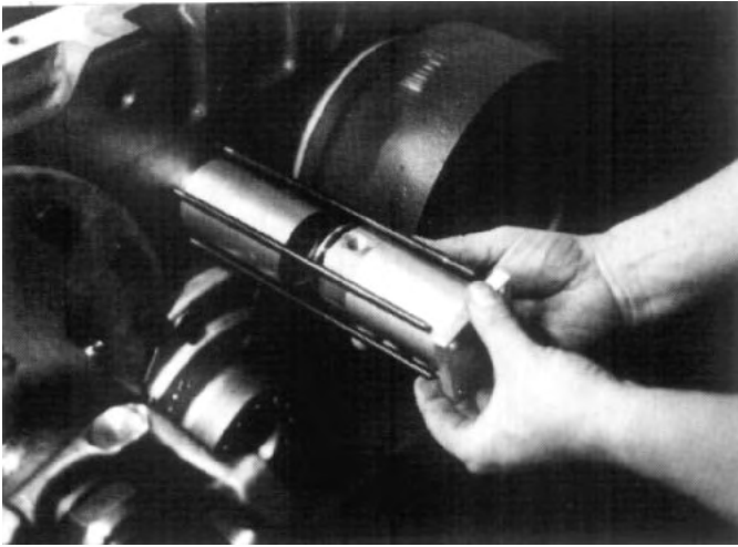
FIG. 6.6-5 If transfer case is not fitted with a neutral shift add the end cap and cap screws at this point, tighten to appropriate torque. Be sure to tighten cap screws evenly. If transfer case has neutral capability, add the long studs and slide the neutral adapter tube with cylinder tube attached into the range shift cylinder. Add stop ring and neutral piston and shift shaft assembly to cylinder. Add end cap with O-ring and tighten nuts on studs evenly to appropriate torque.
