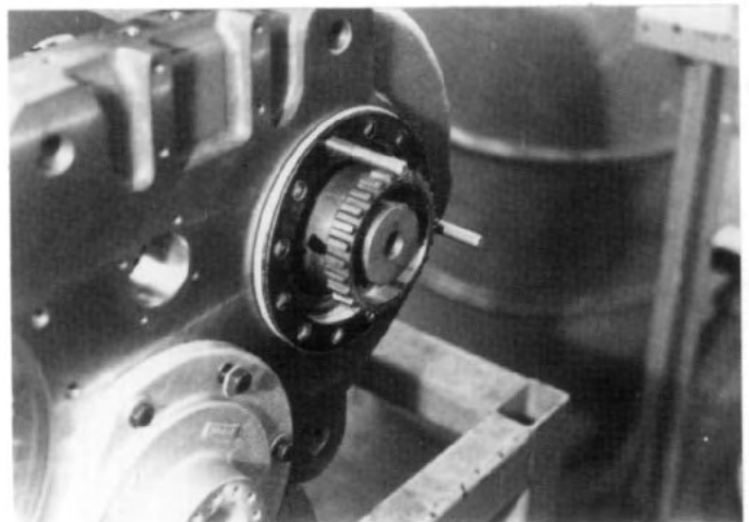
FIG. 6.2-5 Assemble bearing cup, .150 inch shim stack and declutch gear, if required, to rear end of shaft.
