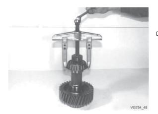
Pull off the rear tapered roller bearing.
