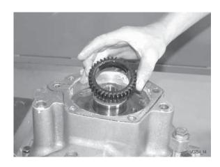
Remove oil pump gear.
