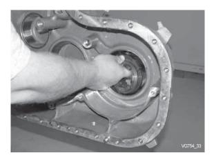
Remove shifting fork and shifting dog sleeve.
