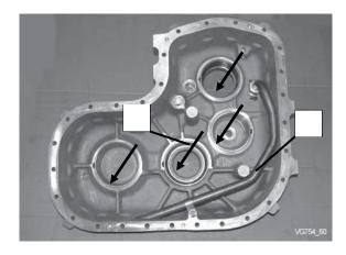
Remove suction line with fitting and spray tube from housing cover (pos. 1).
