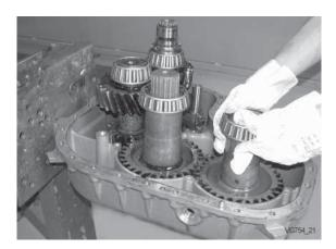
Lift out intermediate shafts and output shaft.
