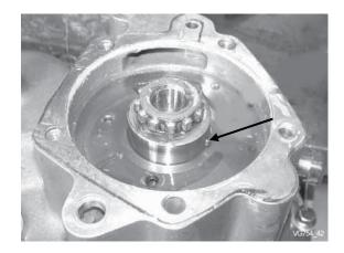
Position drive ball into input shaft with grease.
