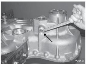
Install sliding sleeve, plug and control switch.
