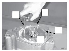
Install oil pump housing and tighten with Allen screws.
