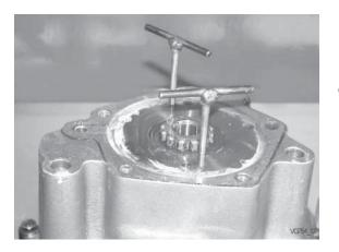
Lift off oil pump housing.
