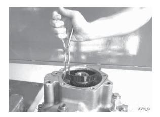
Remove outer oil pump gear.
