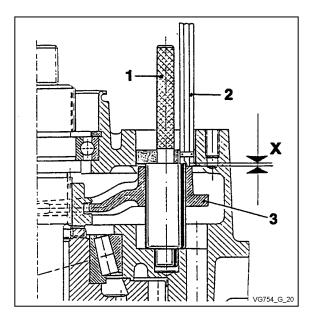
Measure distance **X** between assembly tube (pos. 1) and shift fork (pos. 3).
