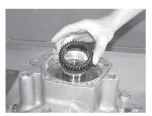
Install oil pump gear on input shaft.
