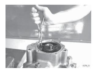
Slide outer pump gear on oil pump gear.
