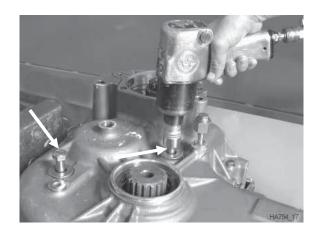
Disassemble anchor screws.
