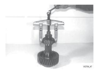
Pull off the rear tapered roller bearing.
