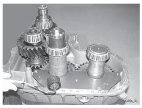
Apply LOCTITE 518 on front housing.
