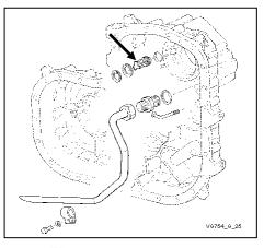
Mount suction line with fitting and spray tube.
