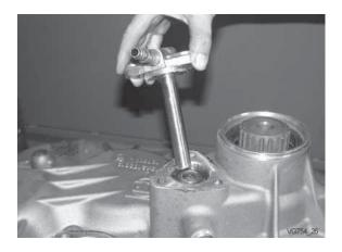
Remove cover and shifting shaft together.
