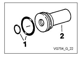
Install O-rings (pos. 1) on piston (pos. 2).
