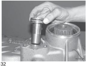
Install shifting piston with seal.
