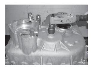
Check rolling torque of the double gear.
