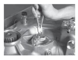
Pull off piston with sealing.
