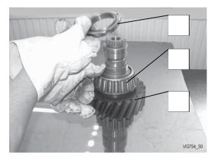
Mount gear (pos. 1) on shaft.
