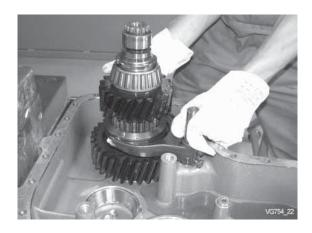
Install input shaft together with shifting fork and shift rod.
