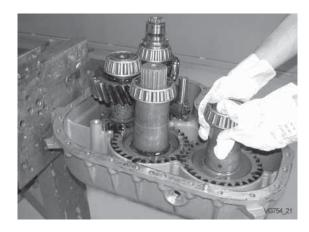
Install intermediate shafts and output shaft.
