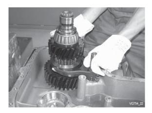
Lift out input shaft together with shifting.
