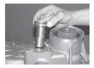
Remove shifting piston with seal.
