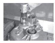
Disassemble oil tube.
