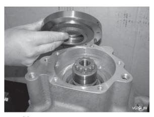
Disassemble oil pump cover.
