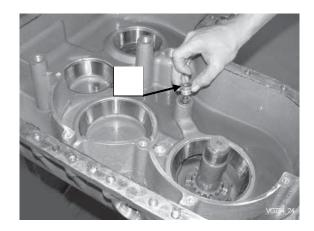
Slide in shaft spring (1) and plug.
