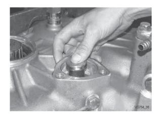
Slide cylinder and seal on shift rod.
