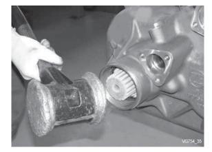
Install input shaft in frozen condition (stored at  $-25^{\circ}$  C in a refridgerator).
