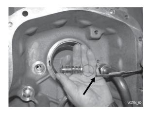
Secure bypass valve with retaining ring.
