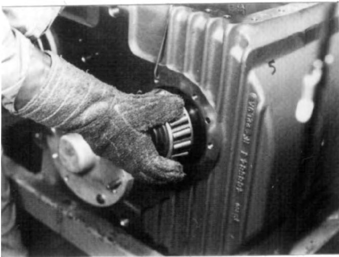
FIG. 6.4-6 Heat remaining shaft bearing cone in heater for approximately 3 minutes and with heat resistant glove slide bearing on shaft to butt against bearing cone under gear.
