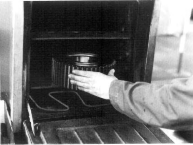
FIG. 6.1-1 Using a domestic electric oven or other suitable heater, place both gears from intermediate shaft inside for approximately 15 minutes. Other heating devices can be used, but gear temperature should not be allowed to exceed 300° F.
