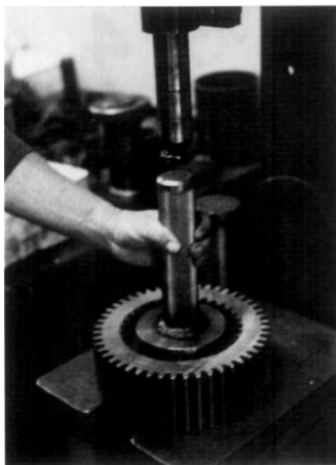
FIG. 6.3-4 Press bearing cups into both gears.
