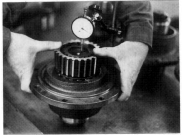
FIG. 6.7-3 Add blanking sleeve or yoke, washer and locknut to output shaft and tighten nut. Mount magnetic base dial test indicator to flange of carrier and check for bearing float on end of shaft as indicated in End Float Adjustment section. End float should be between .003 and .008 inches. Spacer between bearing cones must be machined or changed to one of suitable dimensions to provide the correct end float dimension.
