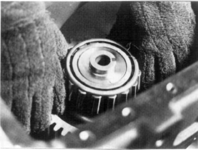
FIG. 6.1-5 Immediately repeat process with the warmed larger bearing cone.
