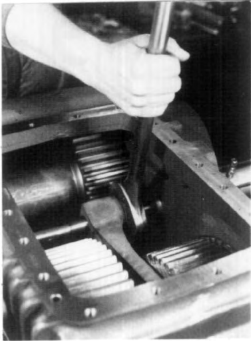
FIG. 6.6-9 With open end wrench tighten nut on shift shaft to the appropriate torque while holding the hexagon key in the end of shift shaft.
