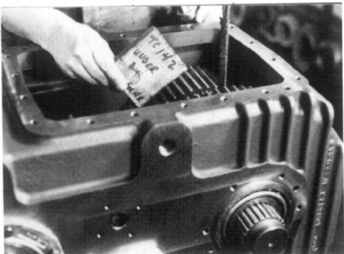
FIG. 6.4-8 Remove wooden block from under gear.
