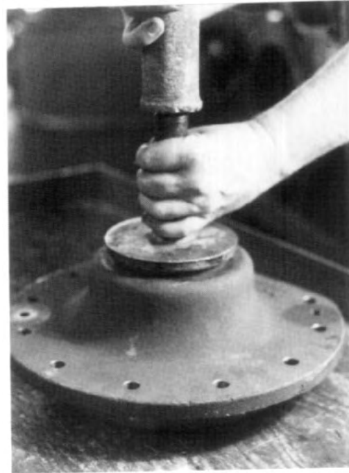
FIG. 6.4-14 Seat oil seal in speed carrier.
