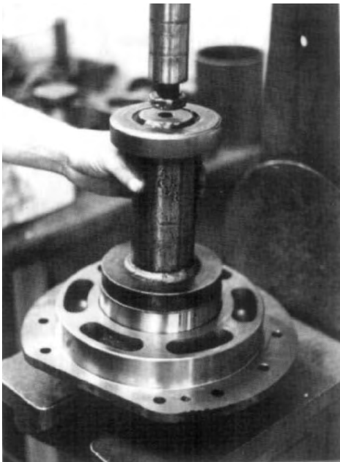
FIG. 6.4-13 Press bearing cup into speed carrier with suitable press.
