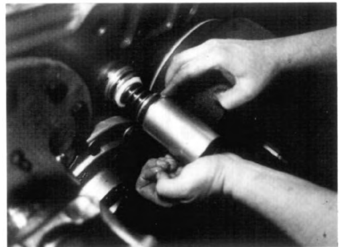
FIG. 6.6-4 Apply a liberal smear of oil and grease slurry to O-ring areas of adapter tube and piston. Presoak the piston felt seal in 30W oil overnight, and wrap into wide groove of piston. While retaining felt in groove with fingers push the cylinder tube onto the piston with the hands. Use caution not to pinch the O-ring seals.
