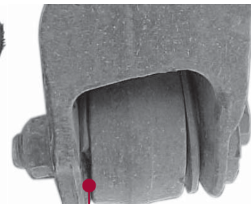
Missing Rubber Flange
