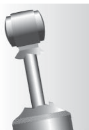
Damaged dust cover and / or shock body
