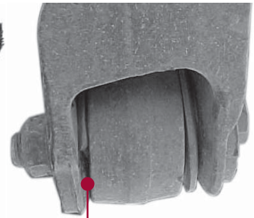
Missing Rubber Flange
