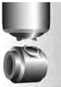
Damaged upper or lower mount
