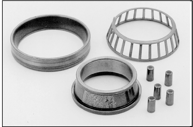
Figure 42 — Tapered Roller Bearing Flaking/Spalling
