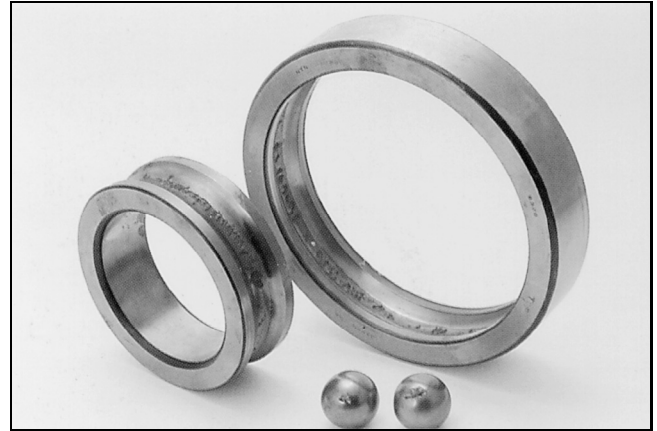
Figure 44 — Ball Bearing Flaking/Spalling
