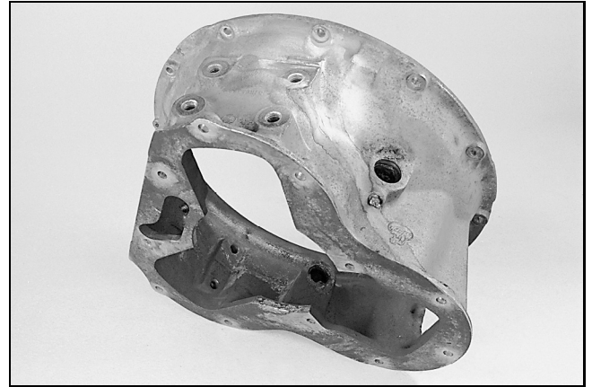
Figure 119 — Cracked Bell Housing (T107 Shown)
