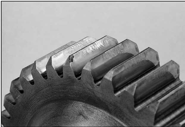
Figure 79 — Damaged Tooth Flank
