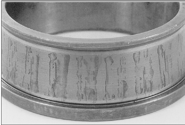
Figure 52 — Water in the Lubricant Caused Rust on the Tapered Roller Inner Race
