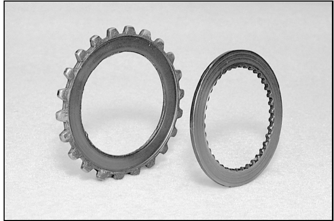
Figure 55 — Thrust Washer Wear
