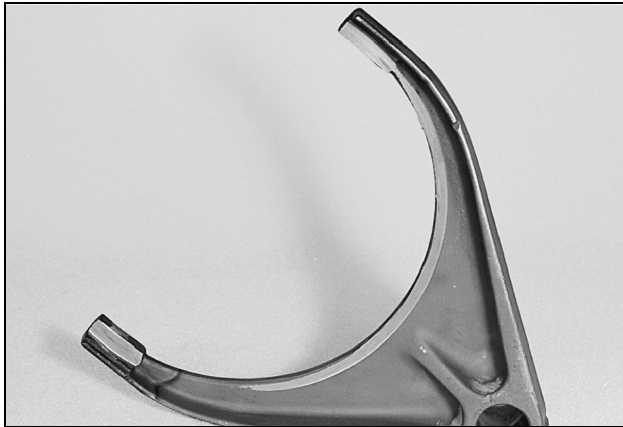
Figure 107 — Worn Shift Fork
