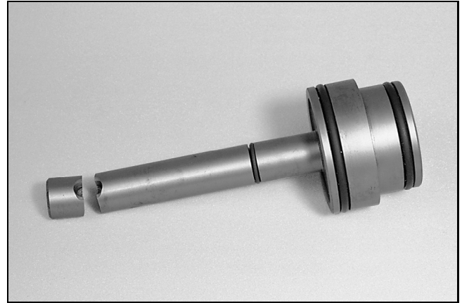
Figure 104 — Range Shift Piston
