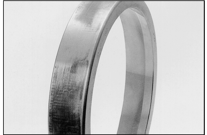
Figure 53 — Fretting and Fretting Corrosion
